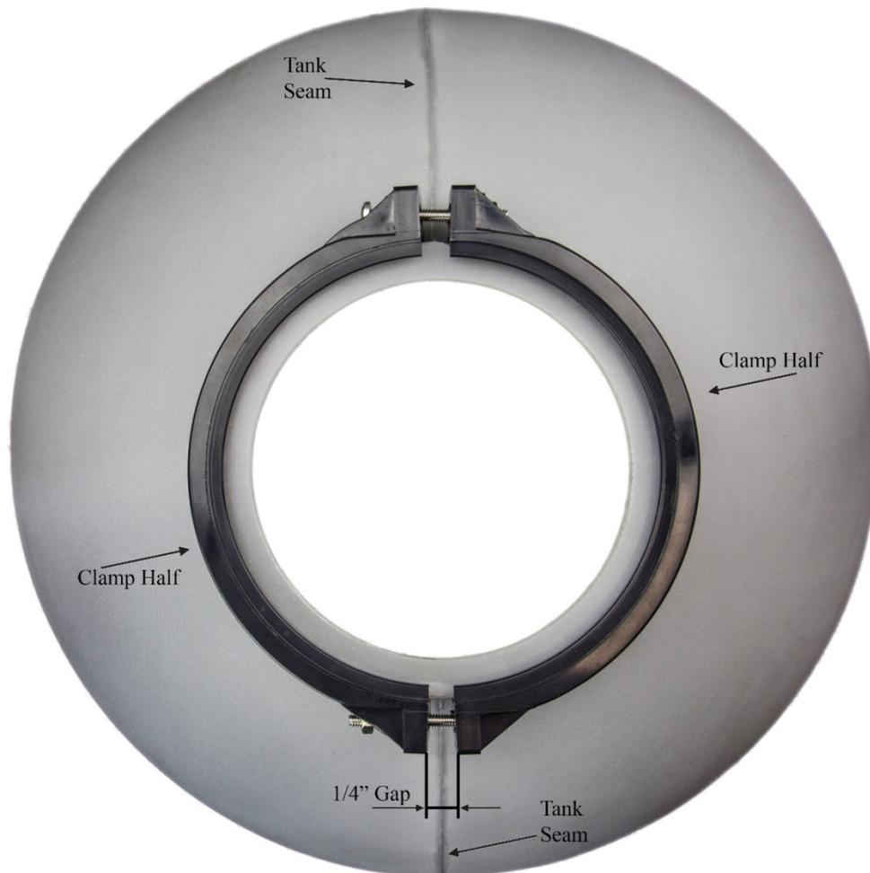
**CAUTION: Over tightening of screws can cause and worsen leaks. Over tightening will ultimately break the clamp. DO NOT USE POWER SCREWDRIVERS TO TIGHTEN CLAMP SCREWS.**
